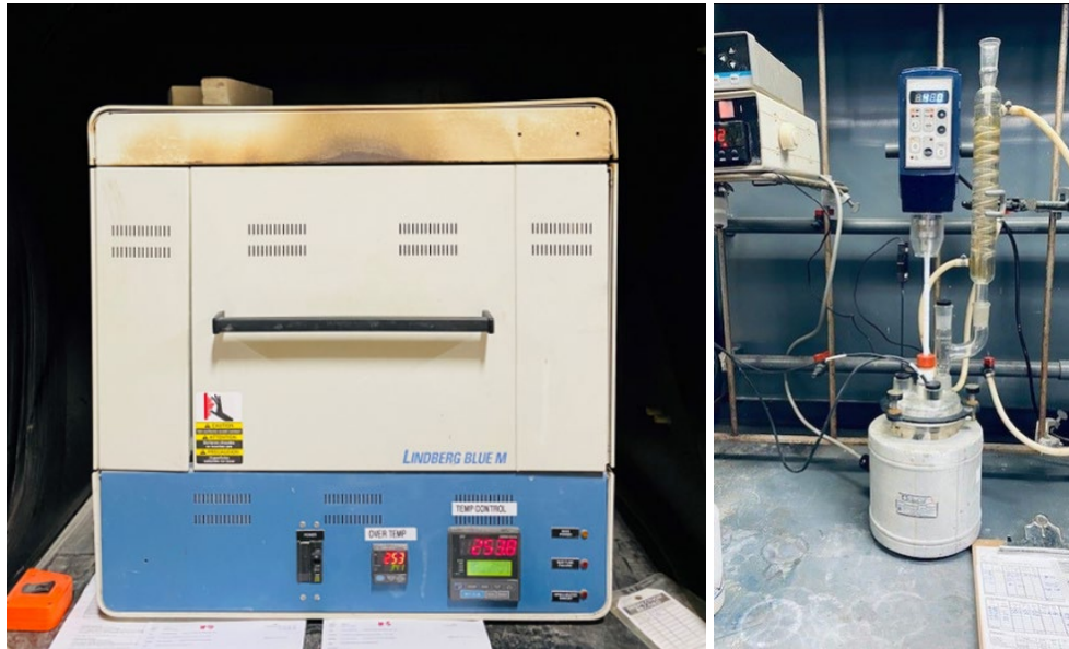
Figure 1: Muffle furnace used for calcination (left) and the water leaching laboratory setup.
