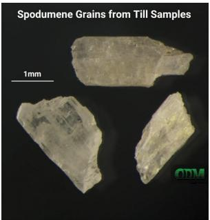
Figure 1 – Spodumene grains from glacial till sampling in the Pontax area.
