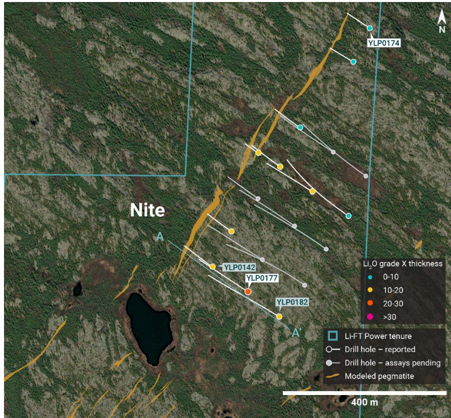
Figure 2 – Plan view showing the surface expression of the Nite pegmatite with diamond drill holes reported in this press release.
