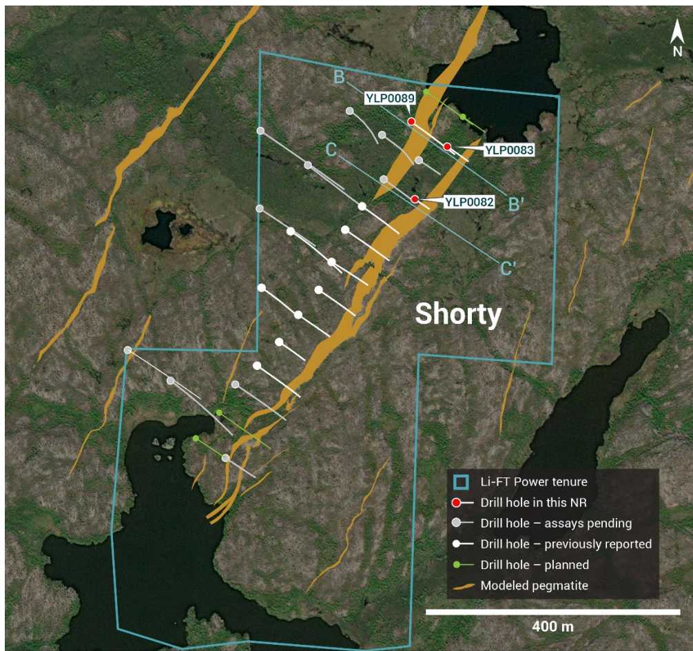
Figure 2 – Plan view showing the surface expression of the Shorty pegmatite with diamond drill holes reported in this press release.
