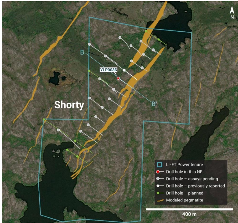
Figure 2 – Plan view showing the surface expression of the Shorty pegmatite with diamond drill hole reported in this press release.
